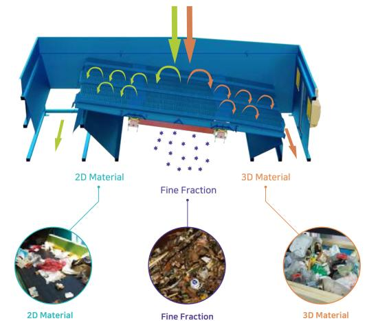
2D materials are conveyed upward the paddle(e.g. Plastic Film, Paper, Textile)
