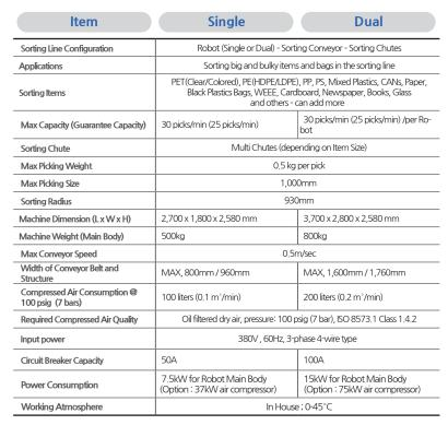
\*The sorting robot is installed on new conveyor at additional cost, and sorting chute and encoder are added on conveyor.
